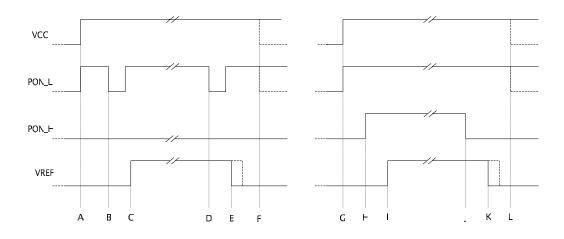
Figure 5.8-1 Typical Power-On & Power-Off Sequences
